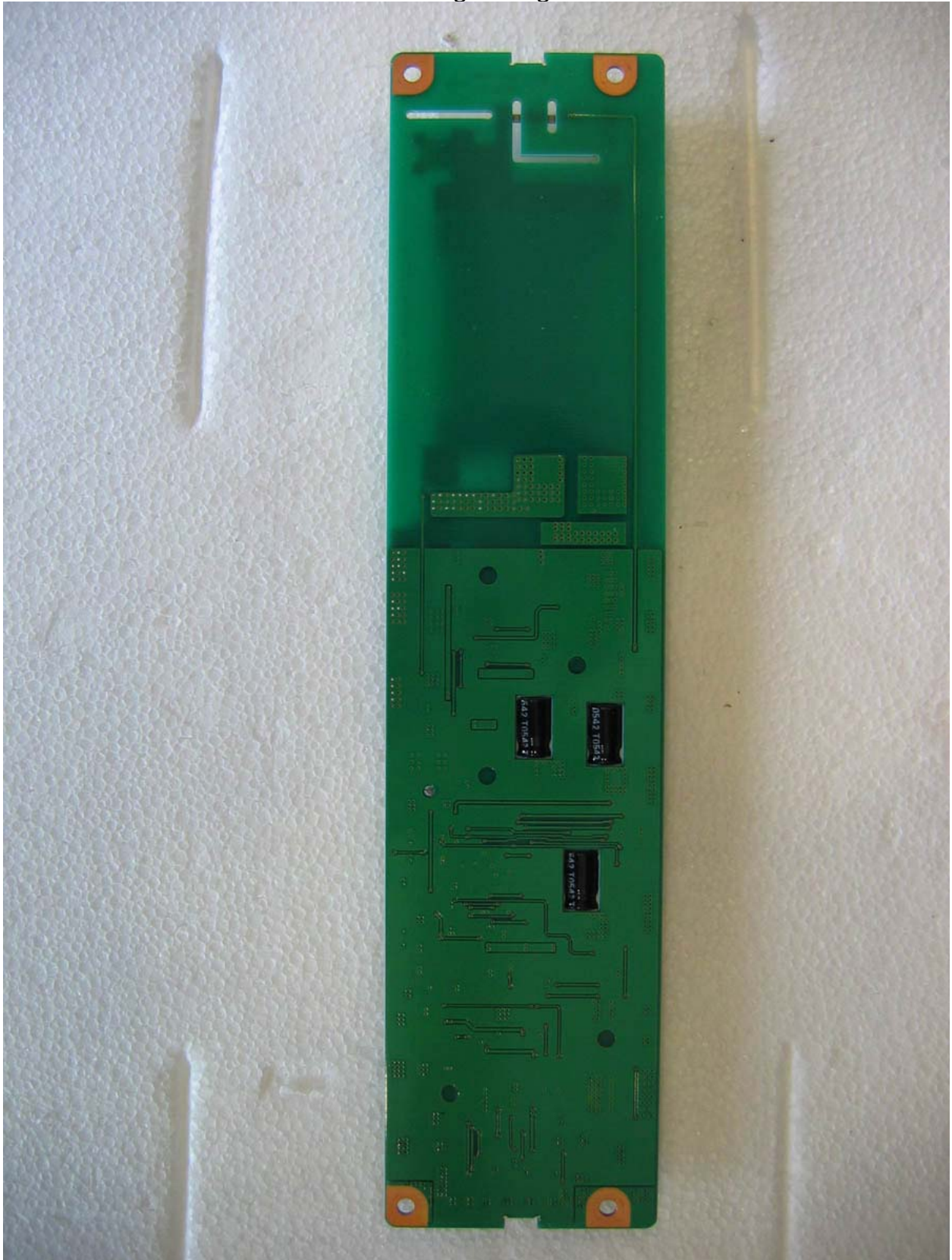
Bottom of high voltage board
