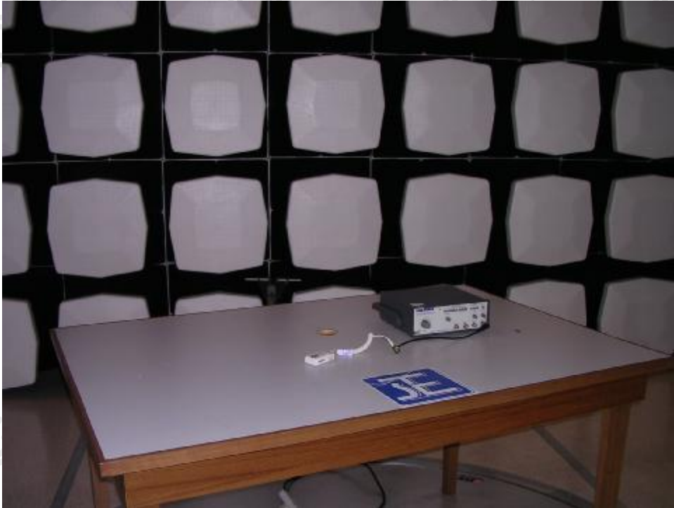
Measurement of Radiated Emission Test Set Up
