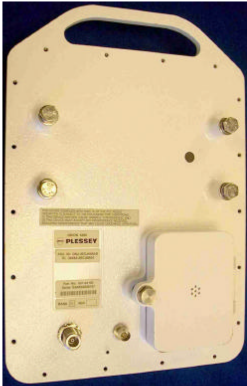
Outdoor RF Unit: Orion 5850 Outdoor RF Unit (Base & Lid sides)
