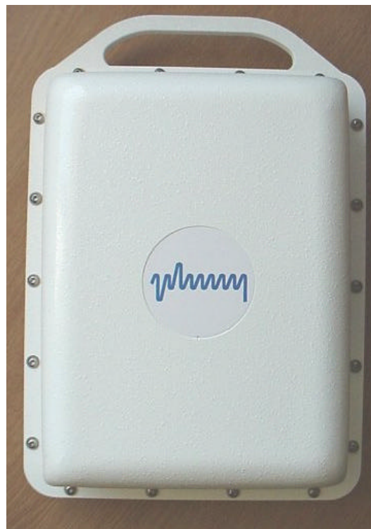
Outdoor RF Unit: Orion 2450 Outdoor RF Unit (Base & Lid sides)
