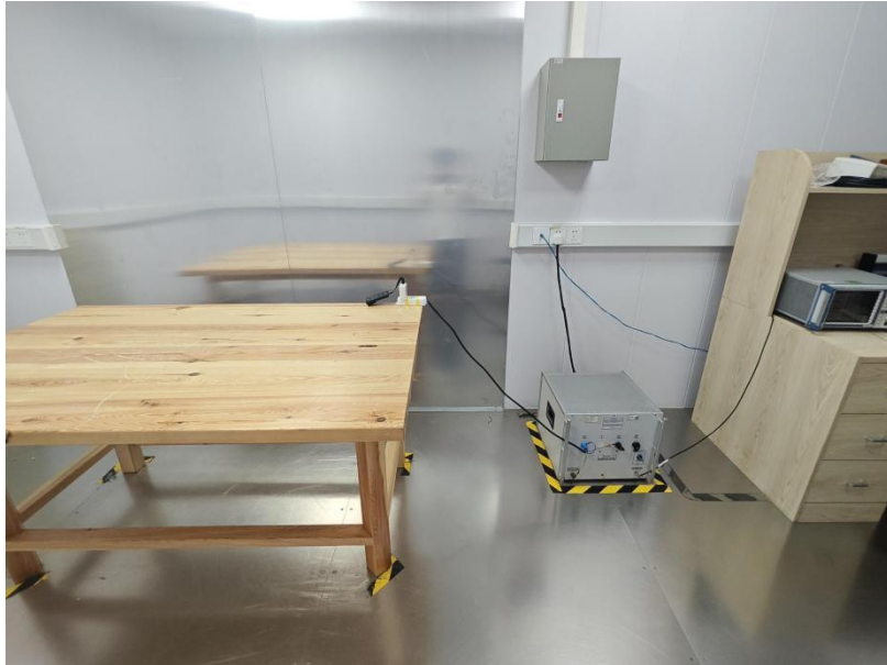
Radiated Spurious Emissions Test Frequency From 9KHz-30MHz
