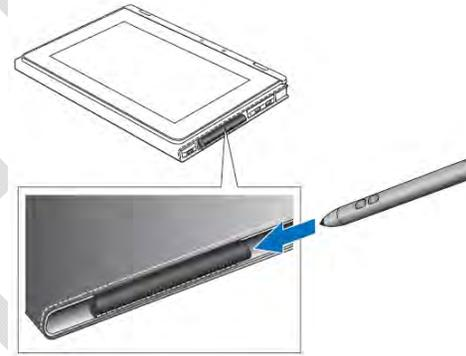
[figure 2-9](#) sleeve alignment for tablet mode
