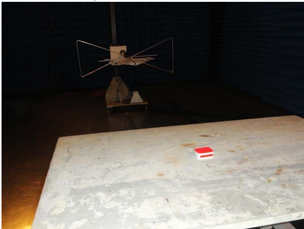
Radiated Emission Test Setup:
