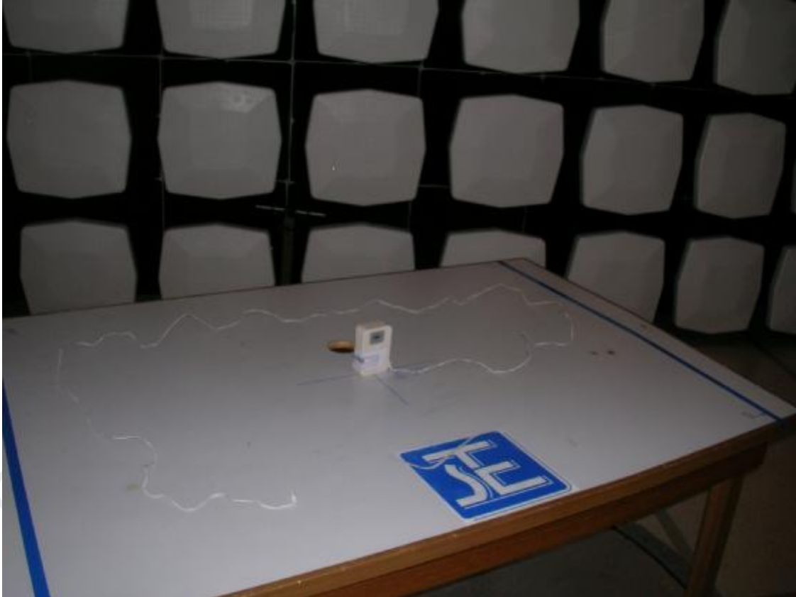
Measurement of Radiated Emission Test Set Up
