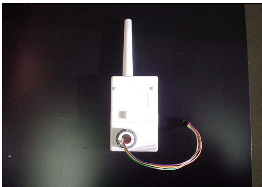
Rear view of the EUT, showing the connection port and the 4-wire cable.
