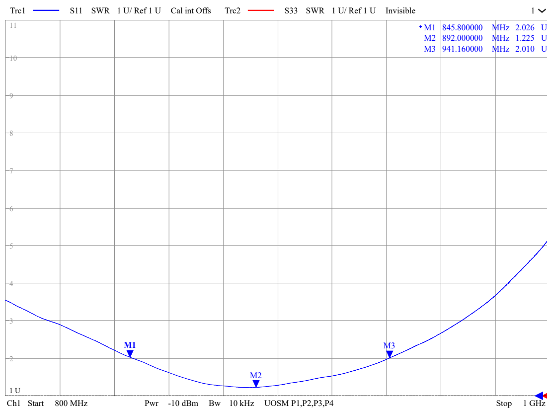
Figure 4-19. SWR Measurement of 892-MHz And Bandwidth at SWR < 2
