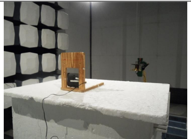
Radiated Emissions (>1GHz) – Rear View
