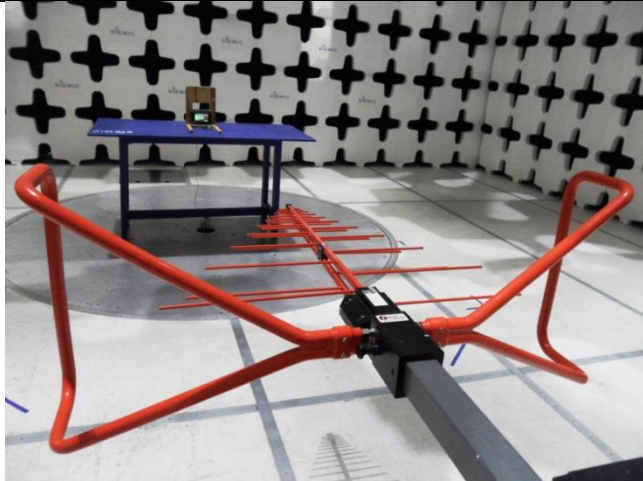
Radiated Emissions (<1GHz) – Front View
