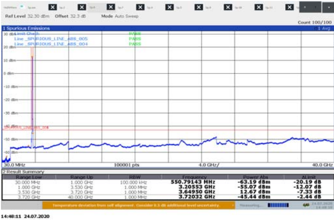
Figure 8.5-21: : Conducted spurious emissions for 20 MHz 3cc high channel 3655 MHz sample plot 30 MHz – 40 GHz
