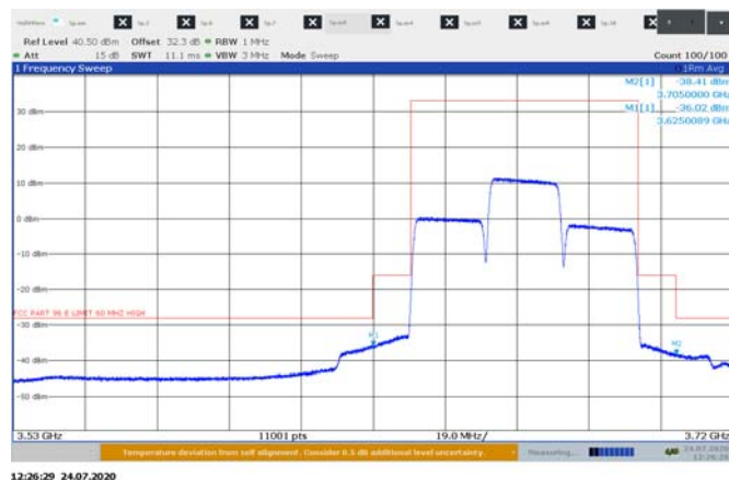
Figure 8.4-21: Emission measurement outside 10 MHz from the SAS assigned channel edge, sample plot for 20 MHz 3cc mid channel
