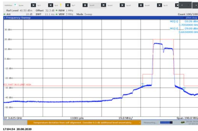
Figure 8.4-5: Emission measurement outside 10 MHz from the SAS assigned channel edge, sample plot for 10 MHz 2cc high channel
