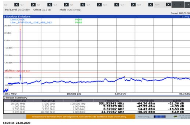
Figure 8.5-6: : Conducted spurious emissions for 10 MHz 3cc low channel sample plot 30 MHz – 40 GHz
