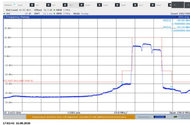
Figure 8.4-11: Emission measurement outside 10 MHz from the SAS assigned channel edge, sample plot for 10 MHz 3cc high channel
