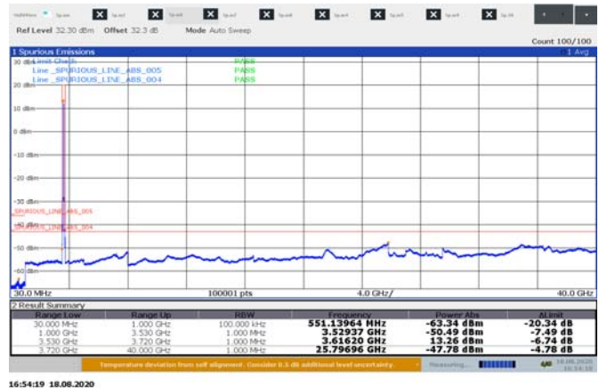
Figure 8.5-12: : Conducted spurious emissions for 20 MHz 2cc mid channel sample plot 30 MHz – 40 GHz
