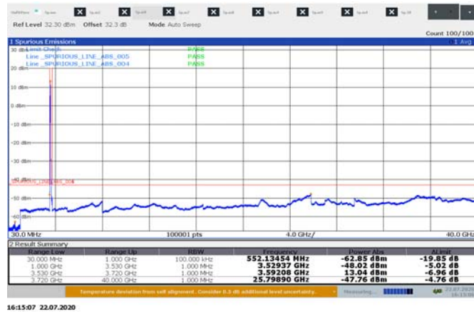
Figure 8.5-16: : Conducted spurious emissions for 20 MHz 3cc low channel sample plot 30 MHz – 40 GHz
