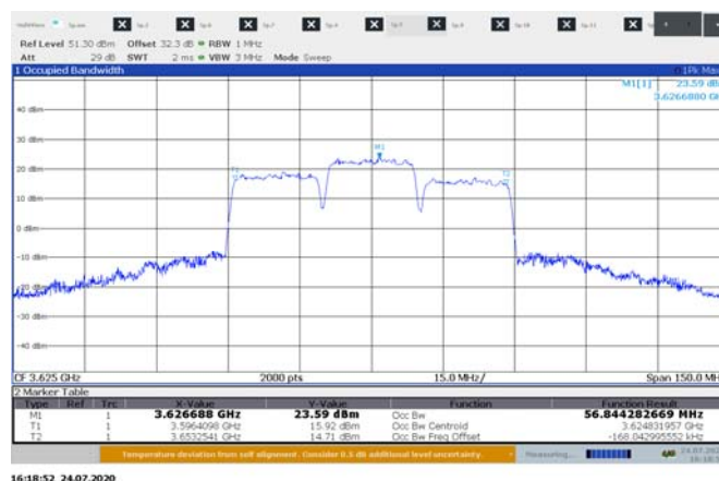
Figure 8.3-4: Occupied bandwidth sample plot for 3CC 20 MHz channel
