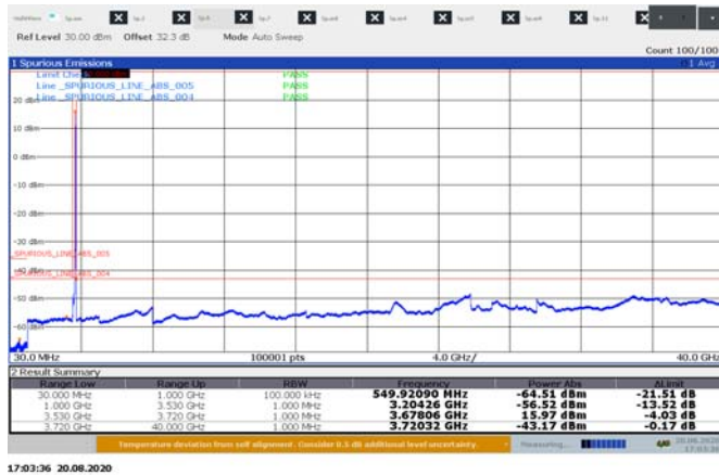
Figure 8.5-3: Conducted spurious emissions for 10 MHz 2cc high channel sample plot 30 MHz – 40 GHz
