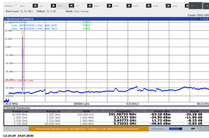
Figure 8.5-18: Conducted spurious emissions for 20 MHz 3cc high channel sample plot 30 MHz – 40 GHz
