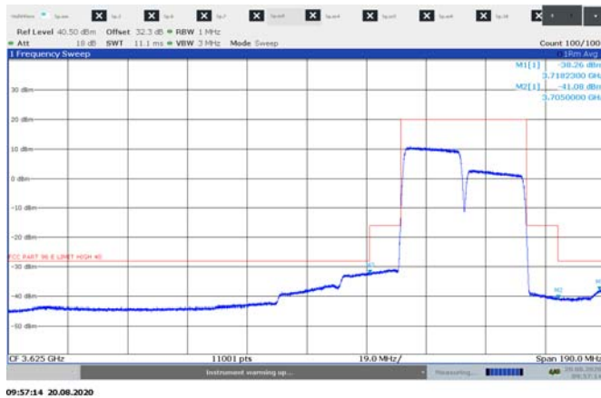
Figure 8.4-17: Emission measurement outside 10 MHz from the SAS assigned channel edge, sample plot for 20 MHz 2cc high channel
