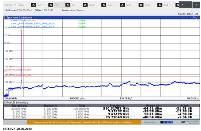
Figure 8.5-2: Conducted spurious emissions for 10 MHz 2cc mid channel sample plot 30 MHz – 40 GHz
