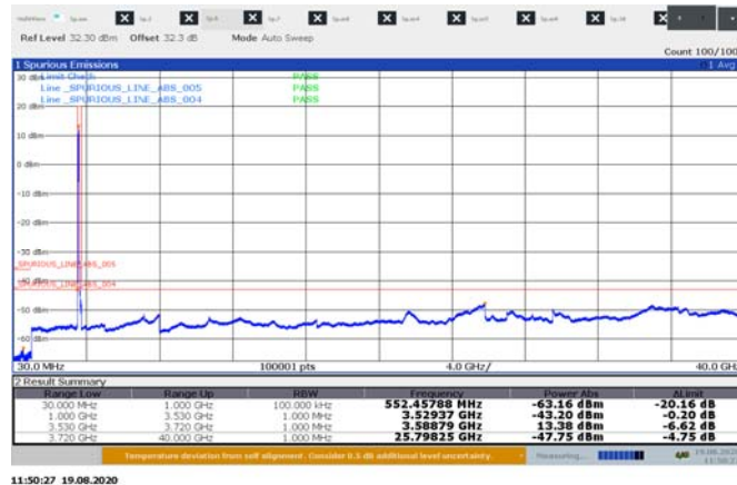
Figure 8.5-11: : Conducted spurious emissions for 20 MHz 2cc low channel sample plot 30 MHz – 40 GHz
