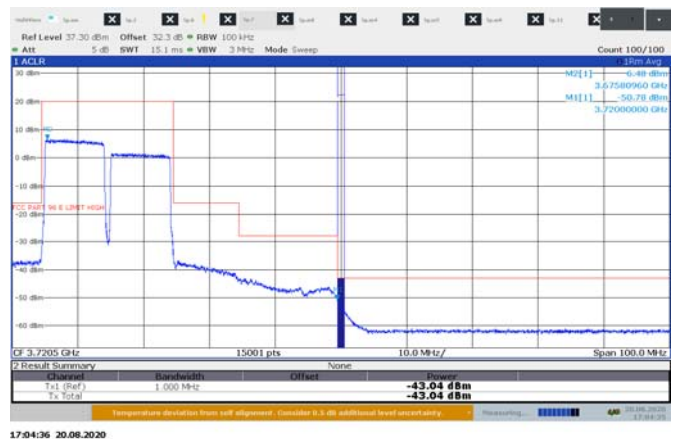
Figure 8.5-5: High Bandedge for 10 MHz 2cc channel at 3720 MHz sample plot
