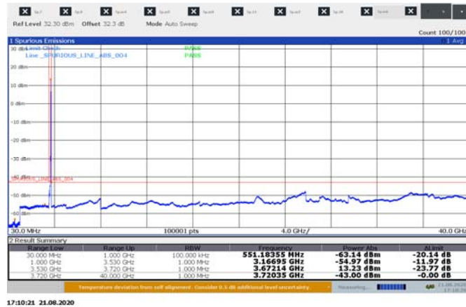
Figure 8.5-8: Conducted spurious emissions for 10 MHz 3cc high channel sample plot 30 MHz – 40 GHz
