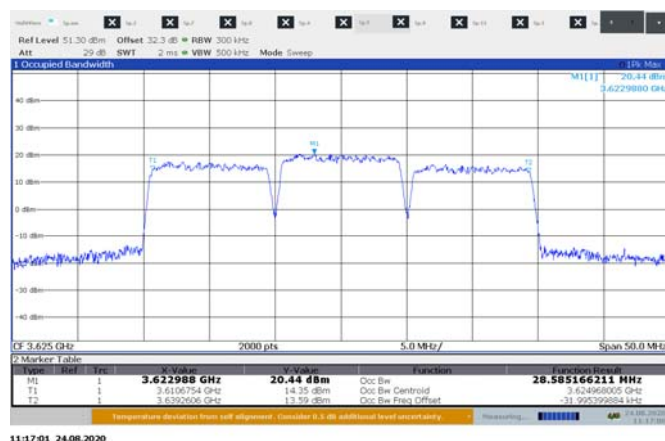
Figure 8.3-3: Occupied bandwidth sample plot for 3CC 10 MHz channel
