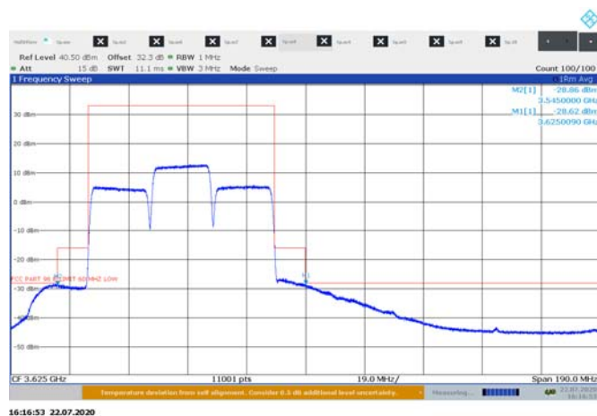
Figure 8.4-19: Emission measurement outside 10 MHz from the SAS assigned channel edge, sample plot for 20 MHz 3cc low channel
