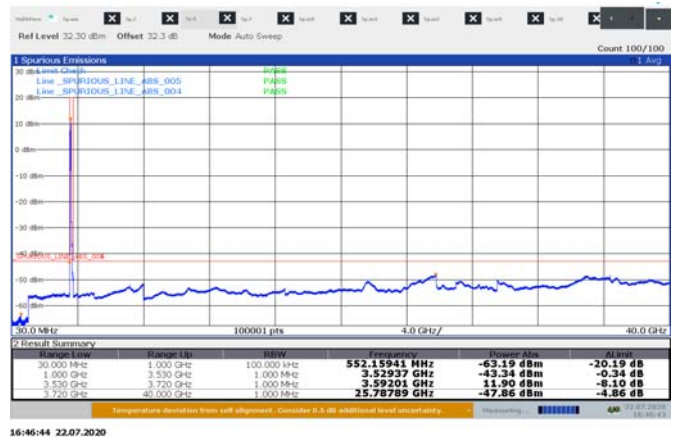
Figure 8.5-17: : Conducted spurious emissions for 20 MHz 3cc mid channel sample plot 30 MHz – 40 GHz
