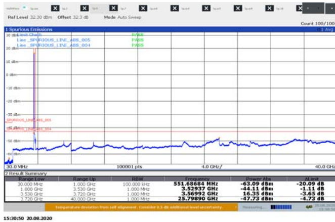
Figure 8.5-1: Conducted spurious emissions for 10 MHz 2cc low channel sample plot 30 MHz – 40 GHz
