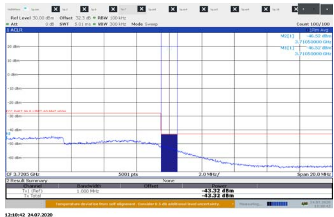
Figure 8.5-20: High Banedge for 20 MHz 3cc channel at 3720 MHz sample plot
