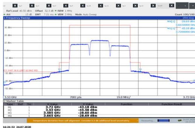
Figure 8.4-21: Emission measurement outside 10 MHz from the SAS assigned channel edge, sample plot for 20 MHz 3cc mid channel
