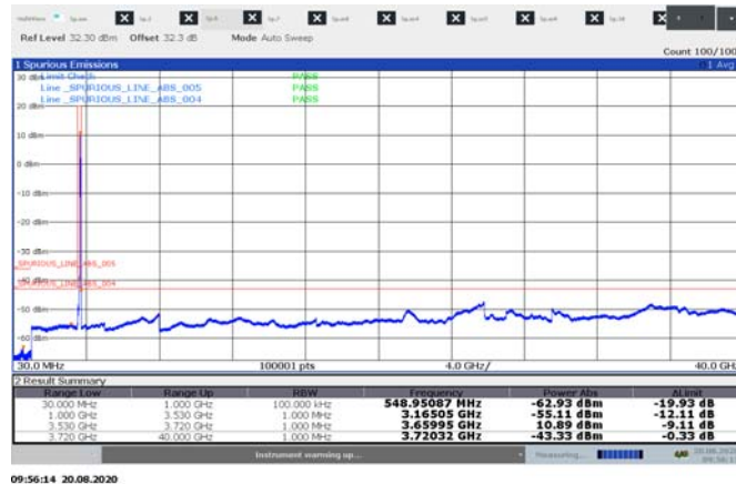
Figure 8.5-13: Conducted spurious emissions for 20 MHz 2cc high channel sample plot 30 MHz – 40 GHz
