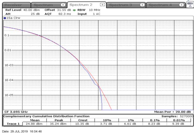
Figure 8.2-1: CCDF sample plot, 1cc 10 MHz channel
