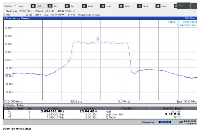
Figure 7.2-8: 26 dB bandwidth, 1CC 10 MHz, sample plot
