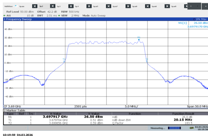
Figure 7.2-9: 26 dB bandwidth, 1CC 20 MHz, sample plot
