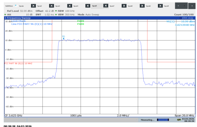
Figure 7.3-6: Conducted band edge, RBW 1 % EBW, 1CC 10 MHz, mid ch
