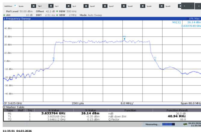
Figure 7.2-11: 26 dB bandwidth, 1CC 40 MHz, sample plot
