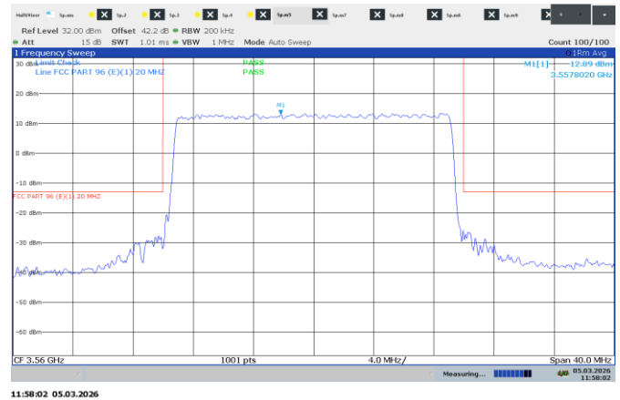
Figure 7.3-16: Conducted band edge, RBW 1 % EBW, 1CC 20 MHz, low ch
