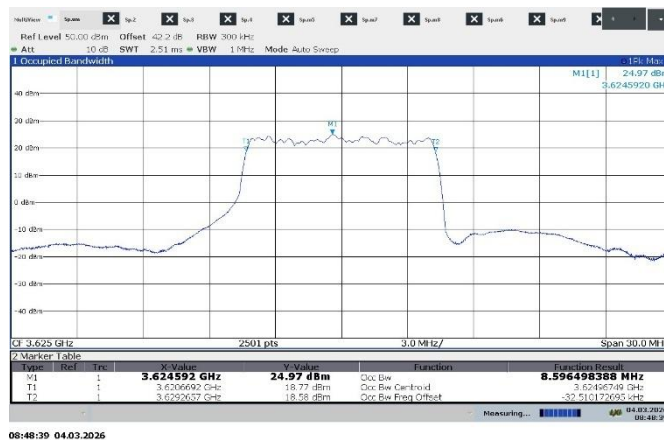
Figure 7.2-1: 99 % occupied bandwidth, 1CC 10 MHz, sample plot
