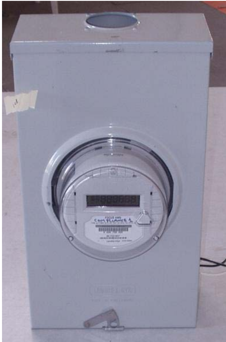
Meter mounted in Socket
