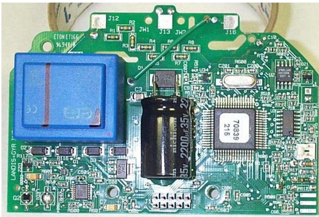
Meter Board – Shield Removed
