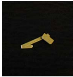
Figure 9 – Formed T-Seal After Installation
