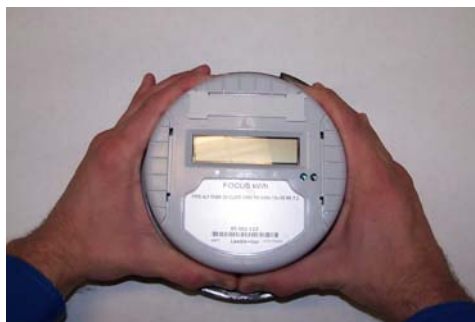
Figure 7 – Removal of Electronics Housing
