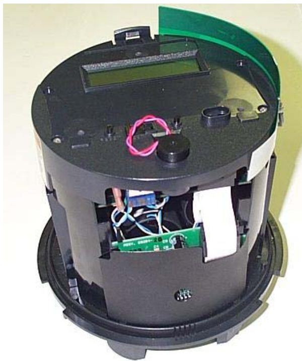
Meter without plastic cover These photos also show the antenna placement.
