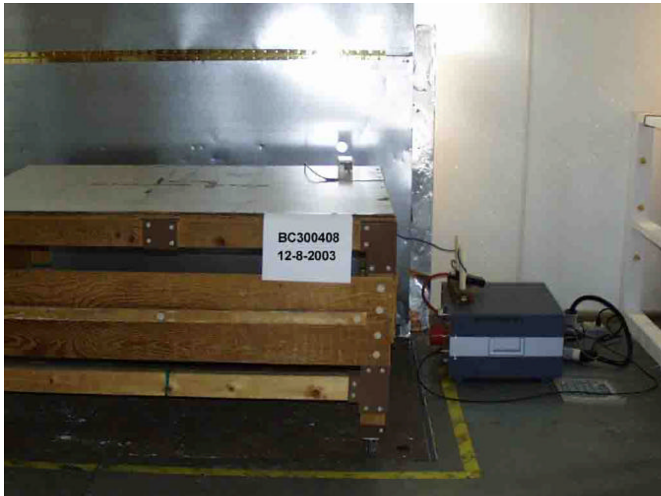
Test-setup photo(s): Conducted Emissions
