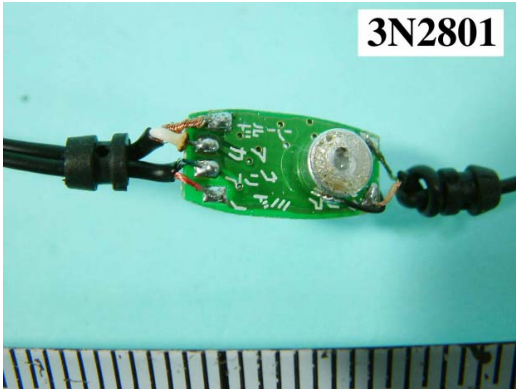
FRONT SIDE OF MAIN BOARD OF EARPHONE
