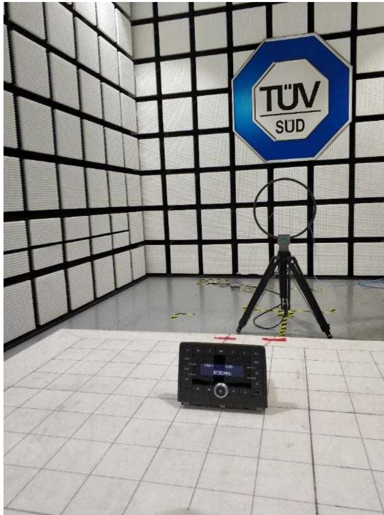
Radiated Emission Setup 9k~30MHz
