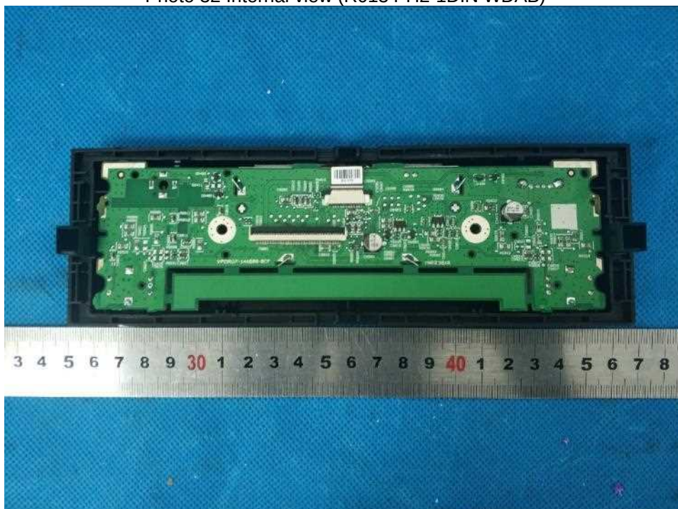
Photo 32 Internal view (R013 PH2-1DIN WDAB)
