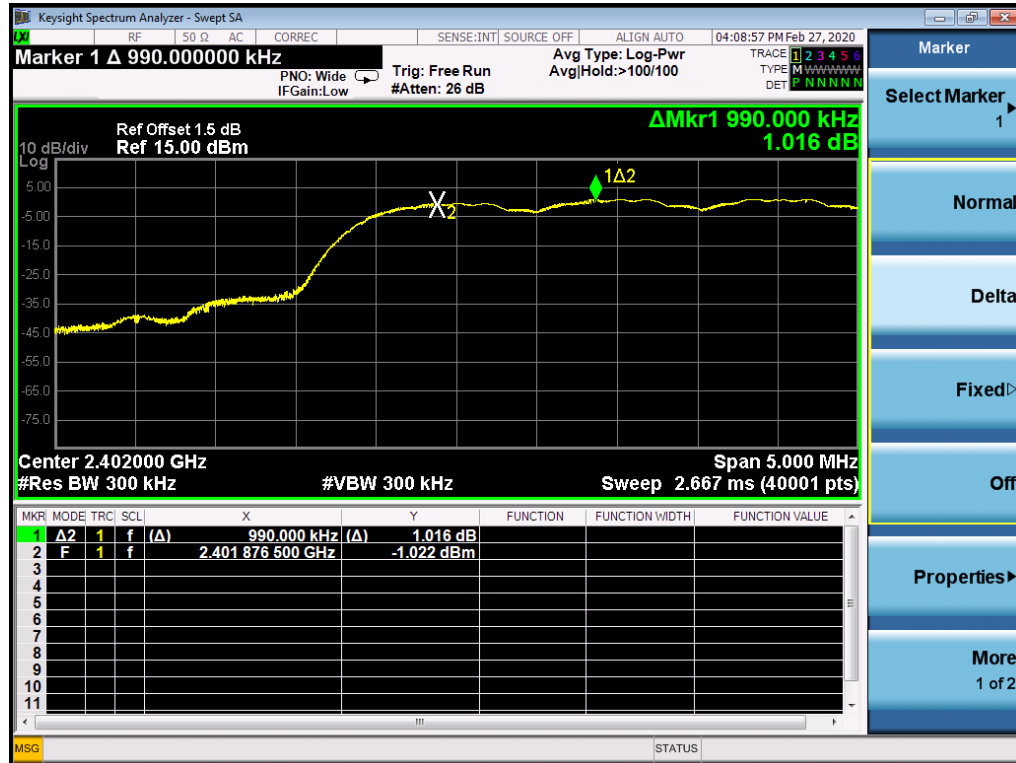
Figure 25: Frequency Separation, TM18, observation Frequency 2402MHz
