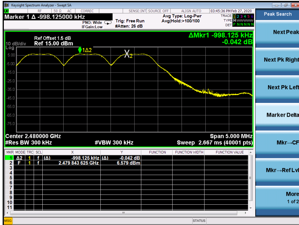
Figure 21: Frequency Separation, TM12, observation Frequency 2480MHz
