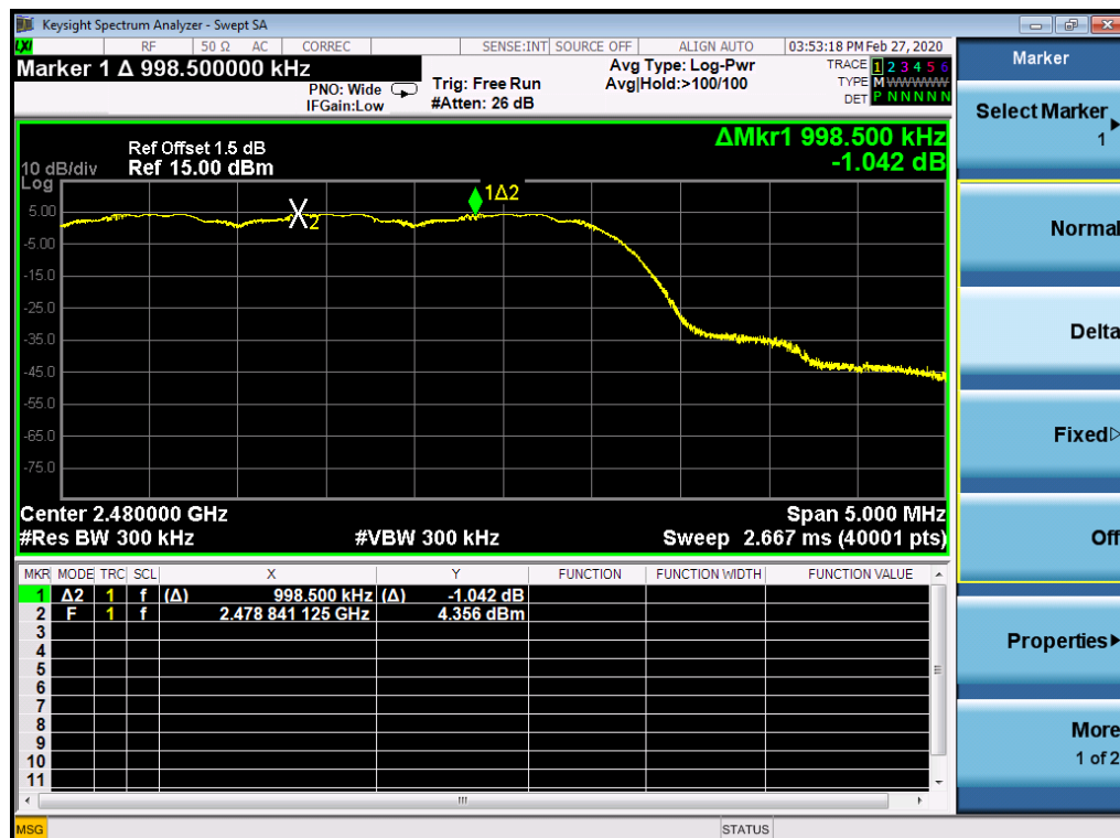
Figure 24: Frequency Separation, TM15, observation Frequency 2480MHz
