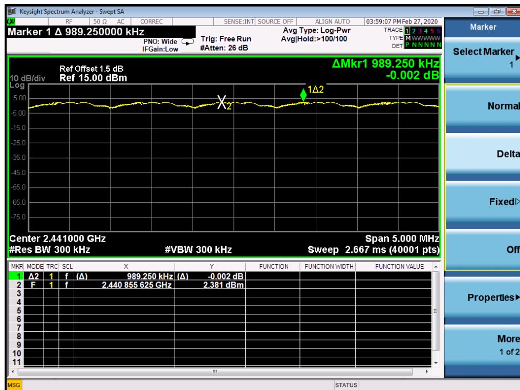
Figure 26: Frequency Separation, TM18, observation Frequency 2441MHz
