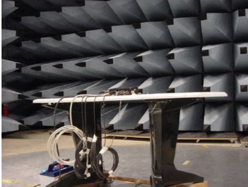
Radiated spurious emission 30 – 1000 MHz
