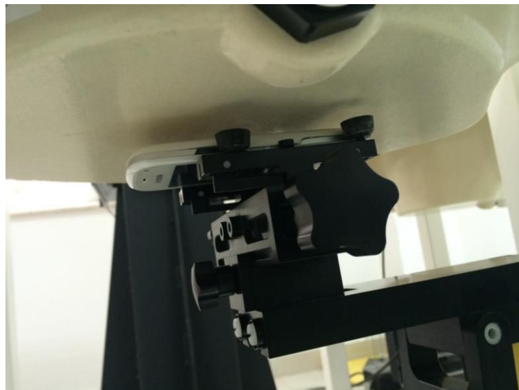
10mm Body-worn Back Side Setup Photo
