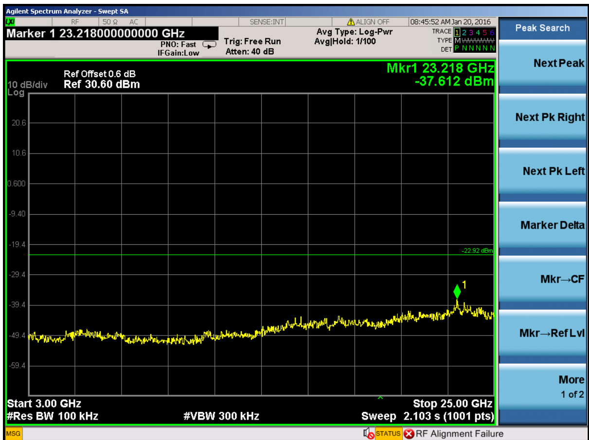
(Plot 4.5.4 C3: Channel 9: 2452MHz @ 802.11n HT40)
