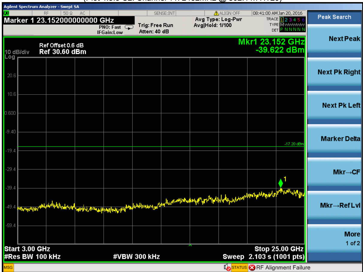
(Plot 4.5.3 C3: Channel 11: 2462MHz @ 802.11n HT20)
