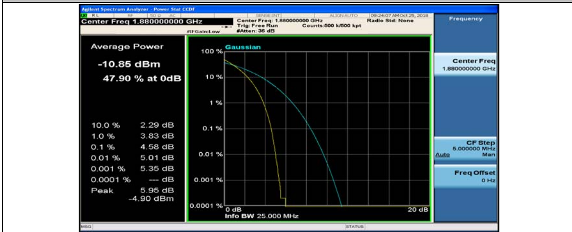
(Channel Bandwidth: 5 MHz)_MCH_QPSK_25RB#0
