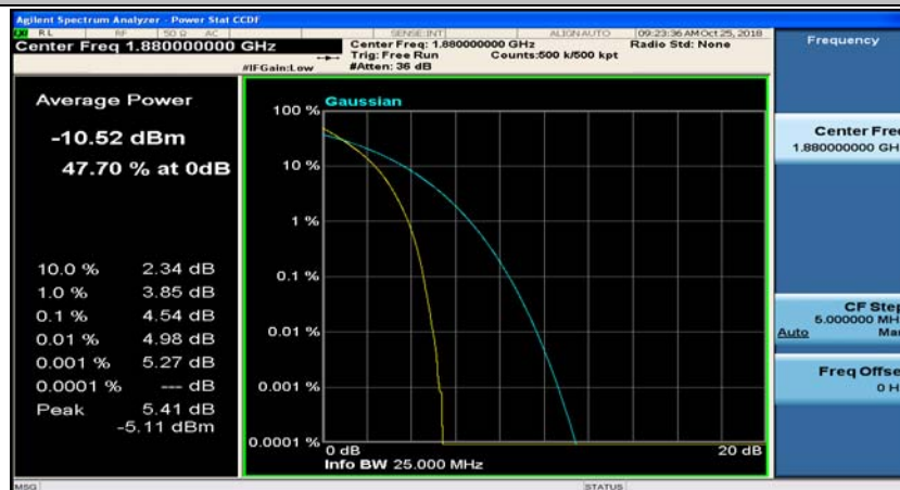
(Channel Bandwidth: 5 MHz)_MCH_QPSK_12RB#13
