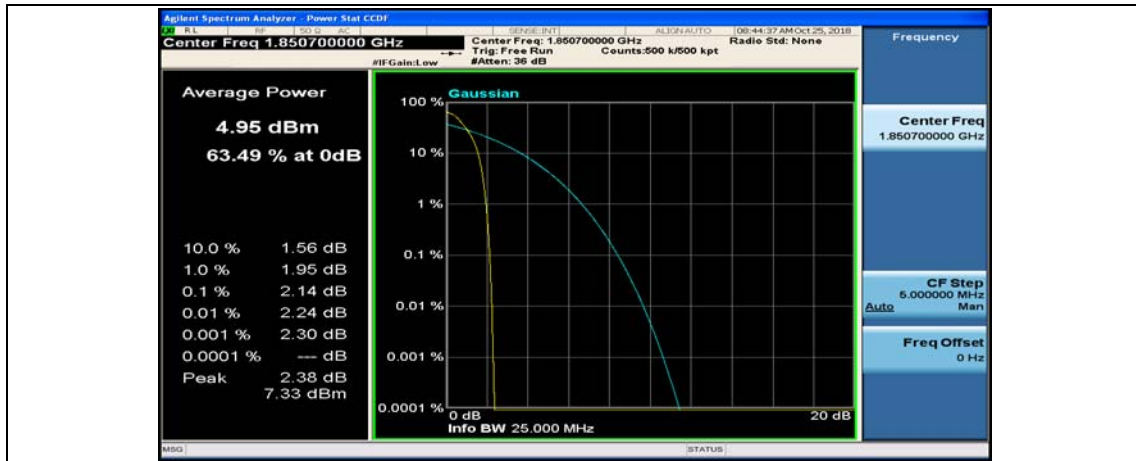
(Channel Bandwidth: 1.4 MHz)_MCH_QPSK_1RB#0
