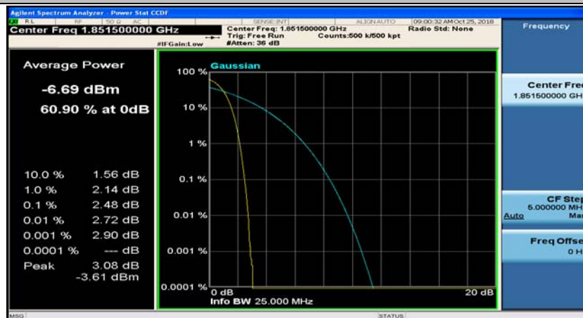
(Channel Bandwidth: 3 MHz)_LCH_QPSK_15RB#0
