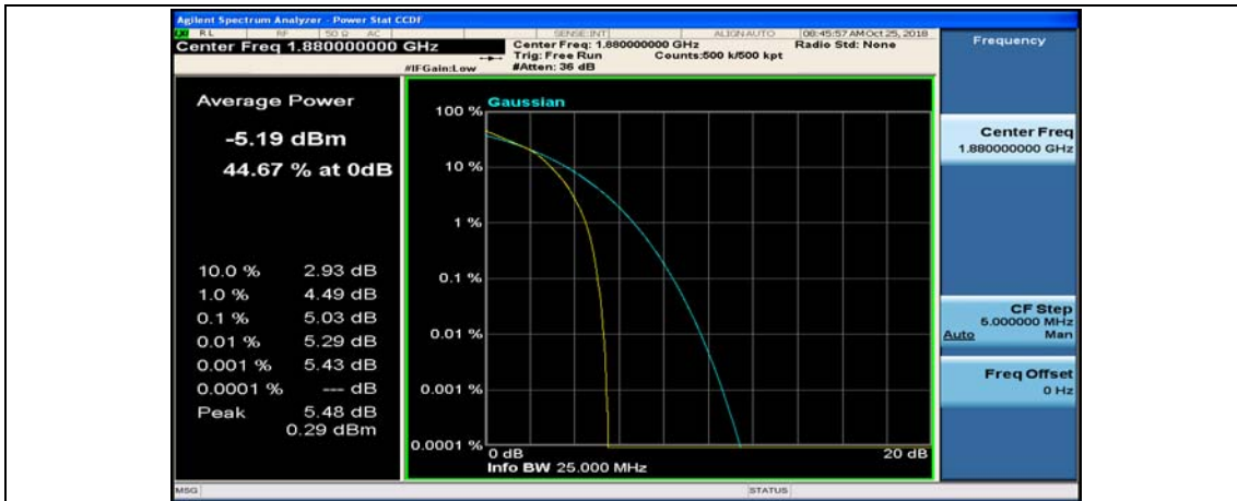
(Channel Bandwidth: 1.4 MHz)_MCH_16QAM_6RB#0
