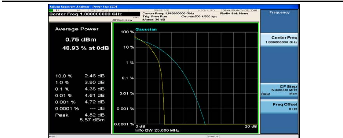
(Channel Bandwidth: 1.4 MHz)_MCH_QPSK_1RB#5
