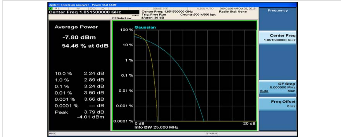
(Channel Bandwidth: 3 MHz)_MCH_16QAM_1RB#0
