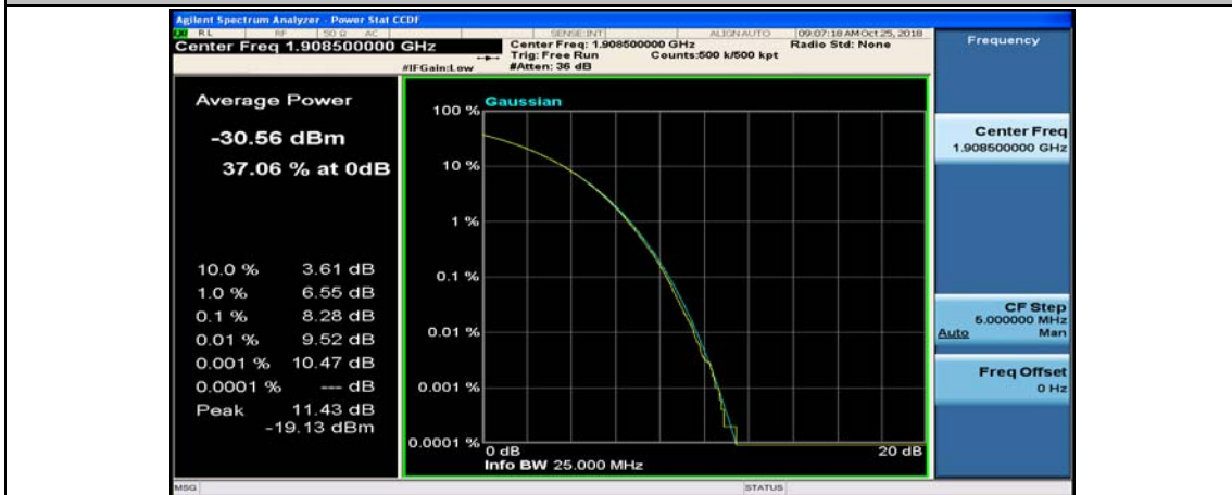
(Channel Bandwidth: 3 MHz)_HCH_16QAM_1RB#7
