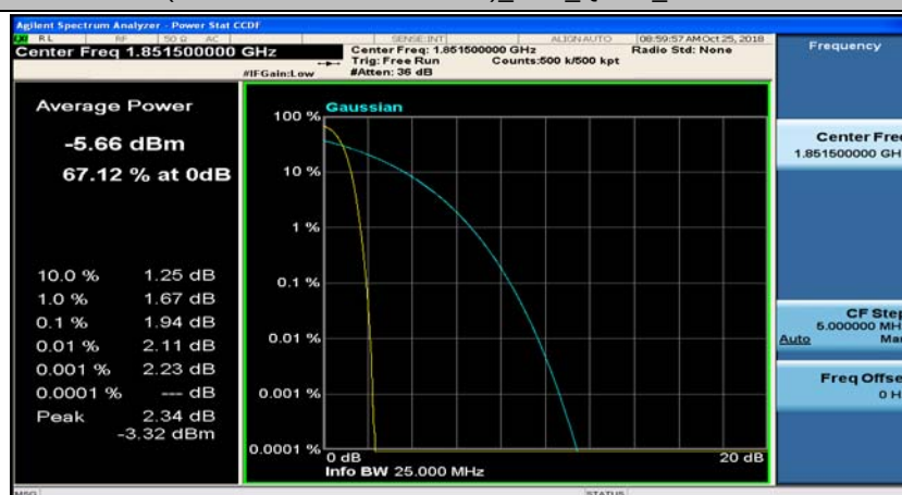
(Channel Bandwidth: 3 MHz)_LCH_QPSK_8RB#0
