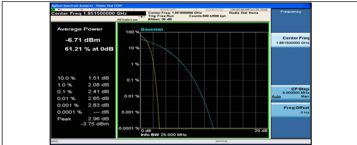
(Channel Bandwidth: 3 MHz)_MCH_QPSK_1RB#0
