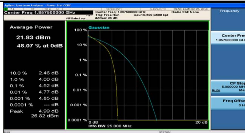
(Channel Bandwidth:15 MHz)_LCH_QPSK_75RB#0
