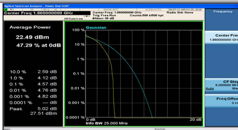
(Channel Bandwidth:20 MHz)_LCH_QPSK_50RB#0
