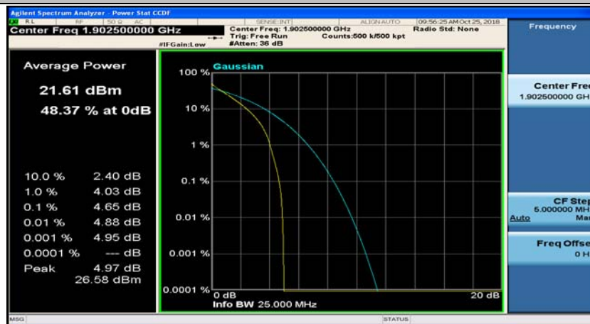
(Channel Bandwidth:15 MHz)_HCH_QPSK_75RB#0
