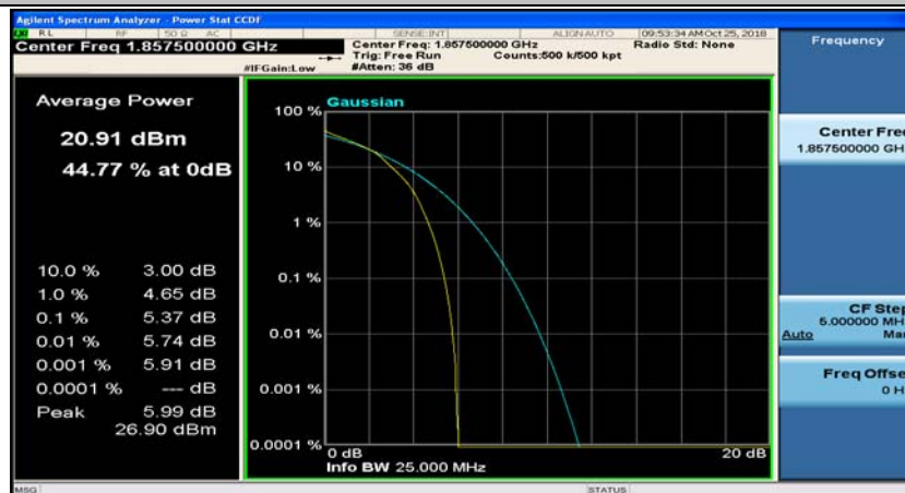
(Channel Bandwidth:15 MHz)_LCH_16QAM_75RB#0
