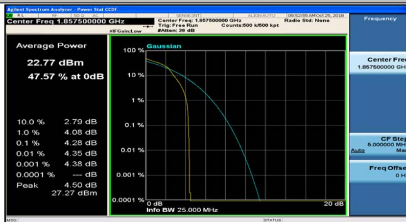
(Channel Bandwidth:15 MHz)_LCH_16QAM_37RB#0
