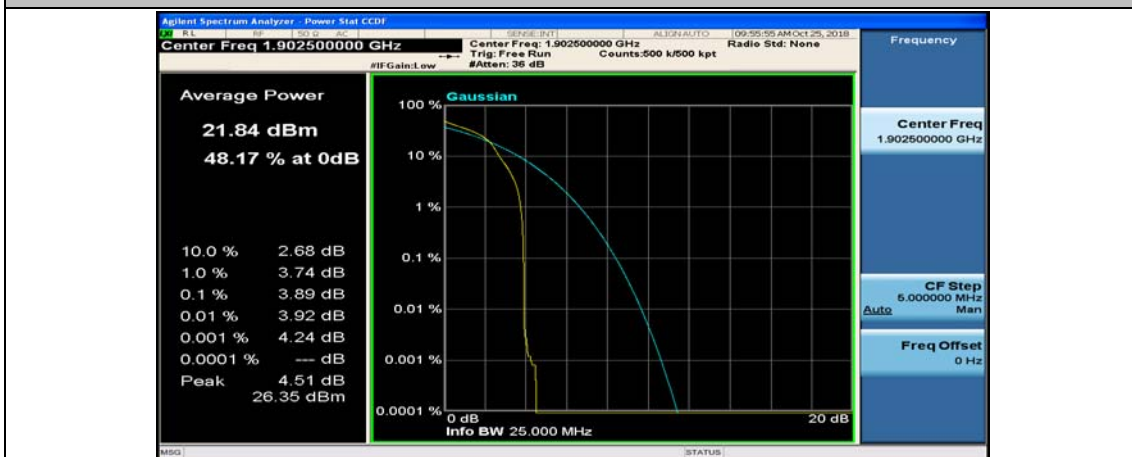
(Channel Bandwidth:15 MHz)_HCH_16QAM_1RB#37
