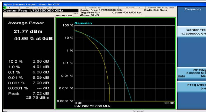
(Channel Bandwidth: 5 MHz)_MCH_16QAM_12RB#13
