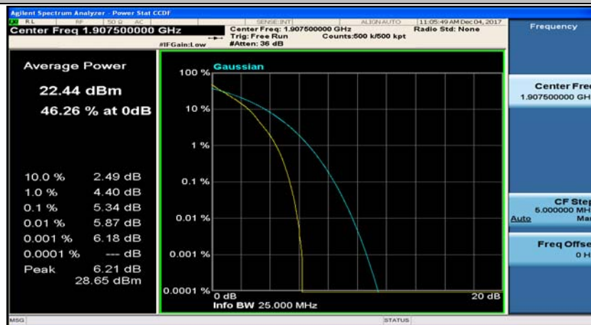
(Channel Bandwidth: 5 MHz)_HCH_QPSK_25RB#0
