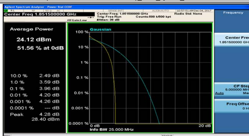
(Channel Bandwidth: 3 MHz)_LCH_QPSK_8RB#0
