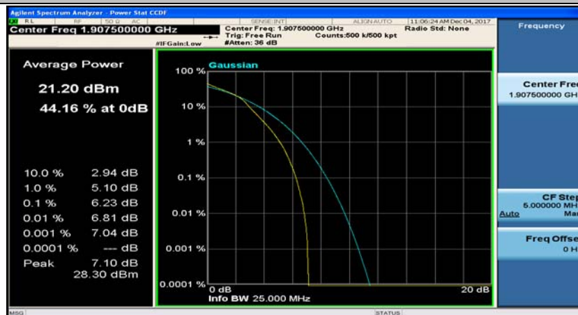
(Channel Bandwidth: 5 MHz)_HCH_16QAM_25RB#0
