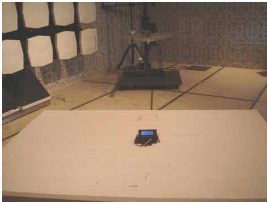
Radiation Emission Test View For 1GHz-25GHz
