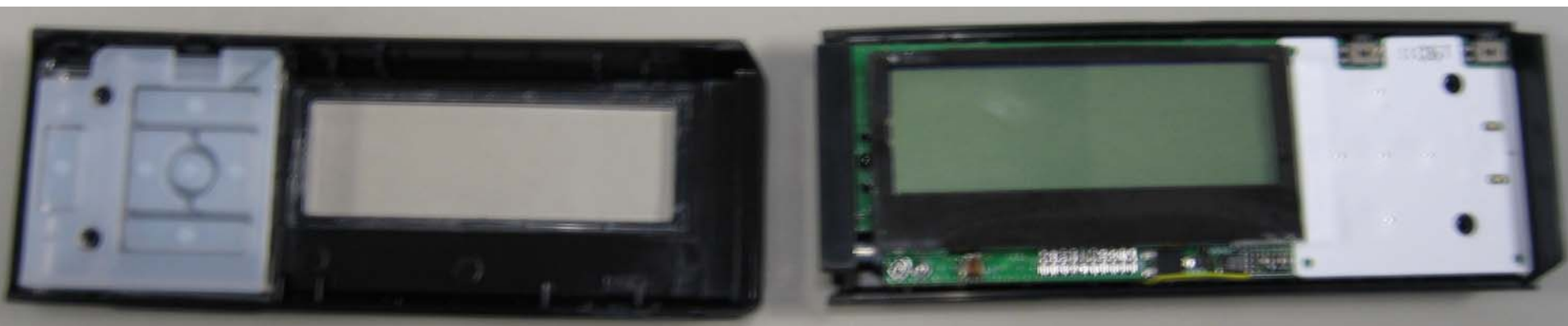
Case Open with PCB Inside
