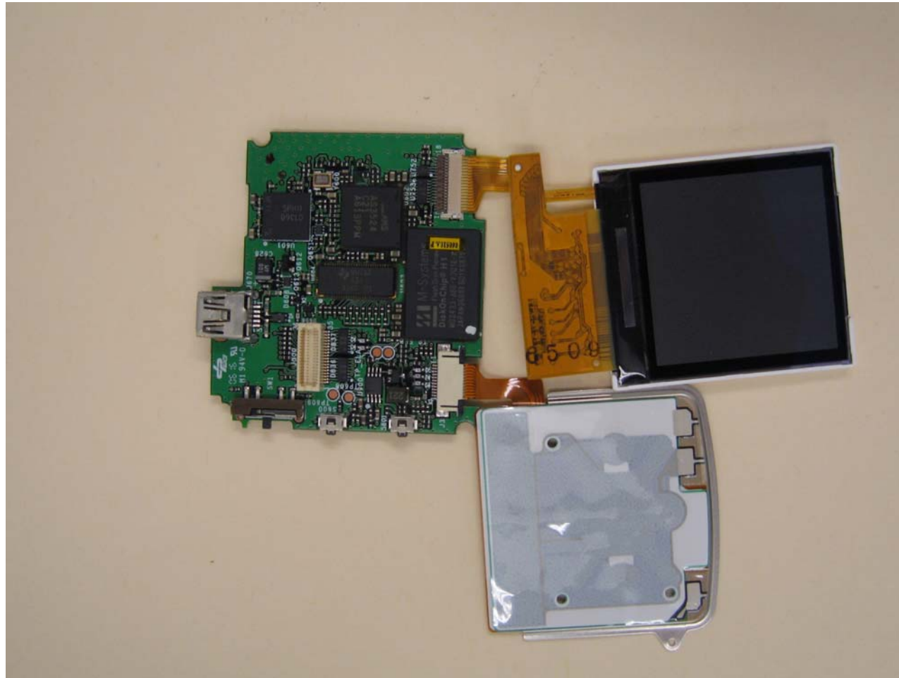
Controller Board - Front
