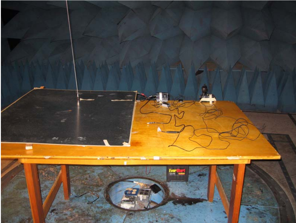
Photo 9 : Car Cradle using FM Direct Adapter (and FM aerial antenna attached to ground plane)
