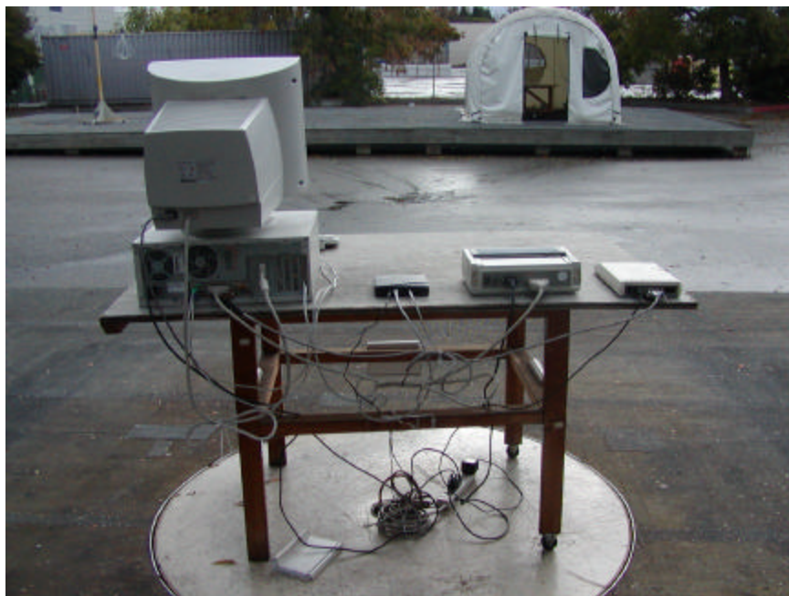
Radiated Emission Setup – Rear View
