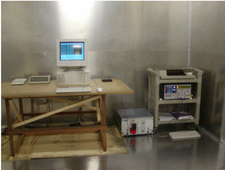
Conducted Emission Setup – Front View
