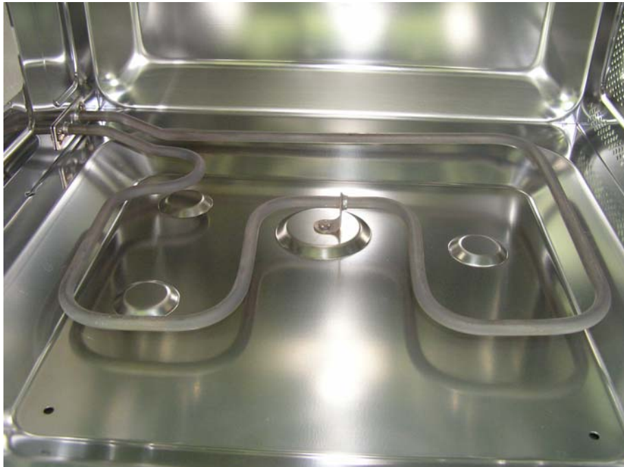
EUT – Heater View
