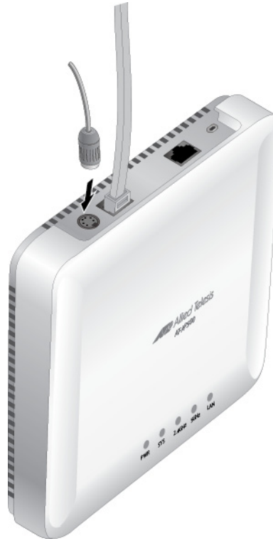
Figure 11. Connecting the Power Cable from the AT-TQ0091 AC/DC Adapter
