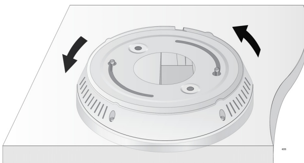
Figure 26. Turning the Access Point to Secure to the Mounting Base
