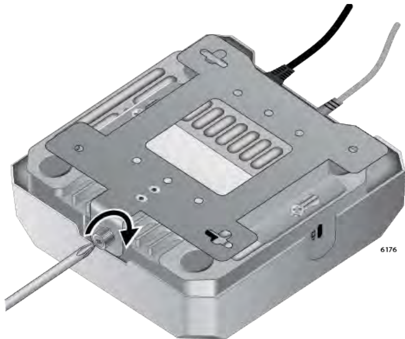
Figure 22. Tightening the Mounting Bracket Thumbscrew
