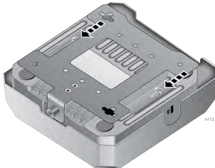
Figure 11. Attaching the Mounting Bracket on the Access Point
