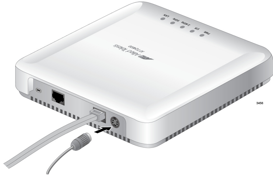
Figure 5. Connecting the Power Cable from the AT-TQ0091 AC/DC Adapter
