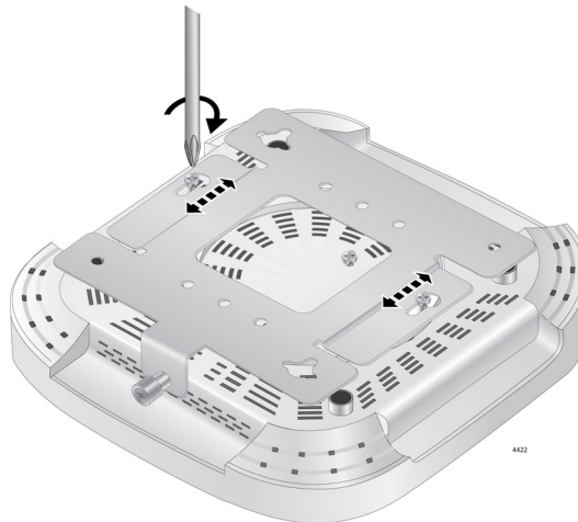
Figure 6. Adjusting the Screws on the Access Point
