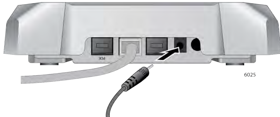
Figure 25. Connecting an AC Power Adapter to the Access Point
