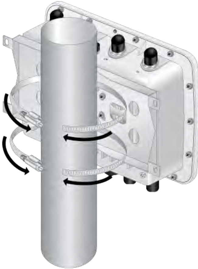
Figure 35. Wrapping the Pole Straps Around the Pole
