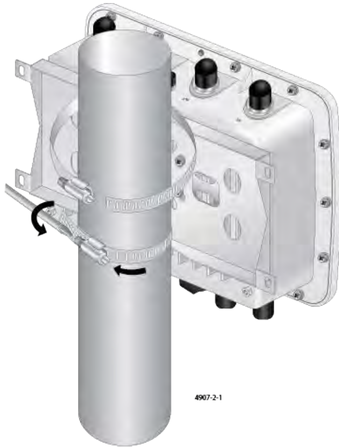
Figure 36. Inserting the Strap Ends into the Screws
