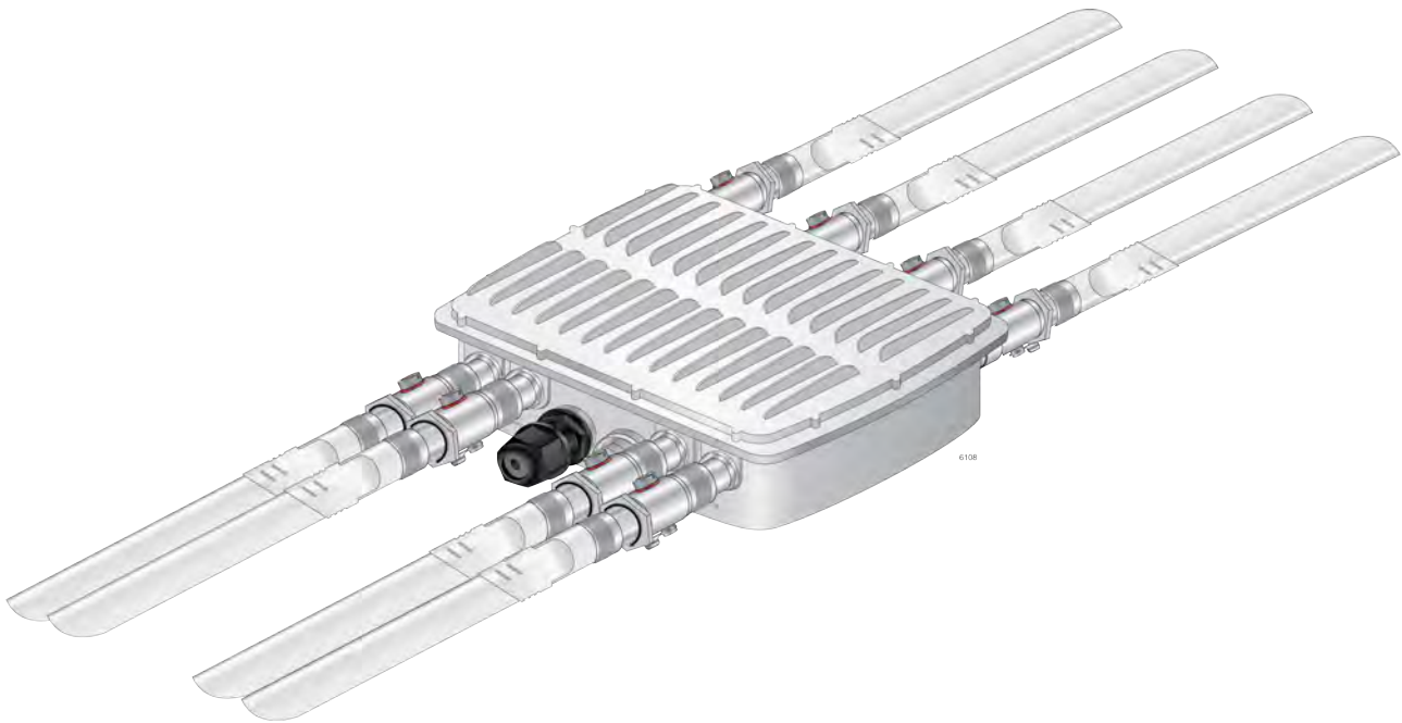
Figure 23. Installing the Antennas to the Access Point
