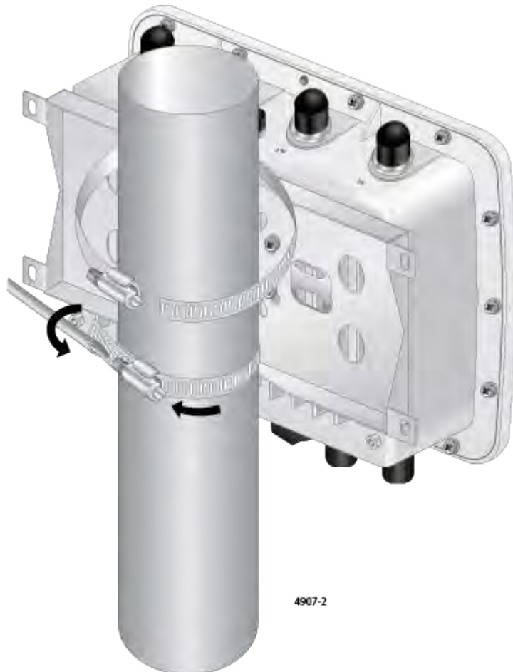
Figure 37. Tightening the Straps
