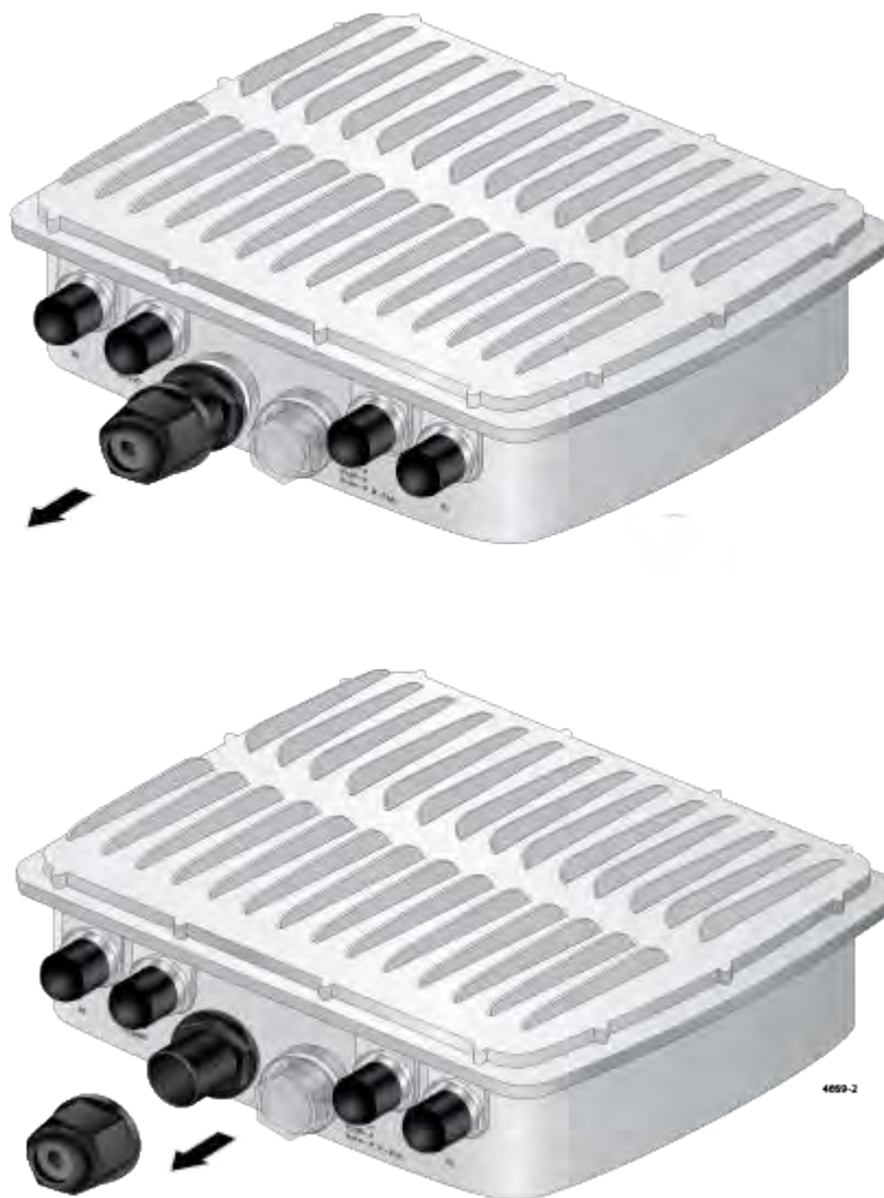
Figure 11. Removing the Cap from the LAN Port
