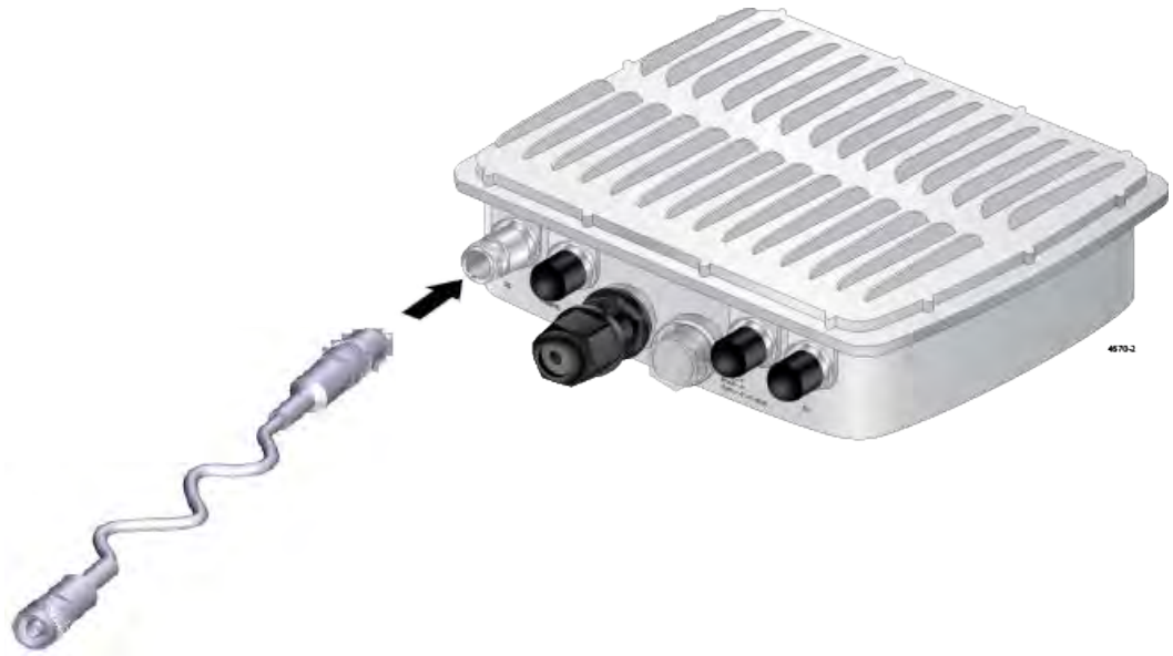
Figure 45. Attaching the cable to an Antenna Connector
