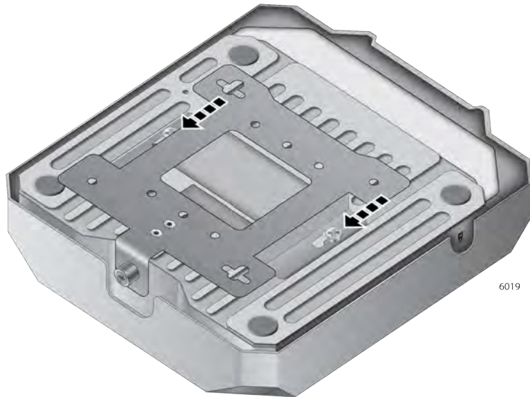
Figure 15. Attaching the Mounting Bracket on the Access Point
