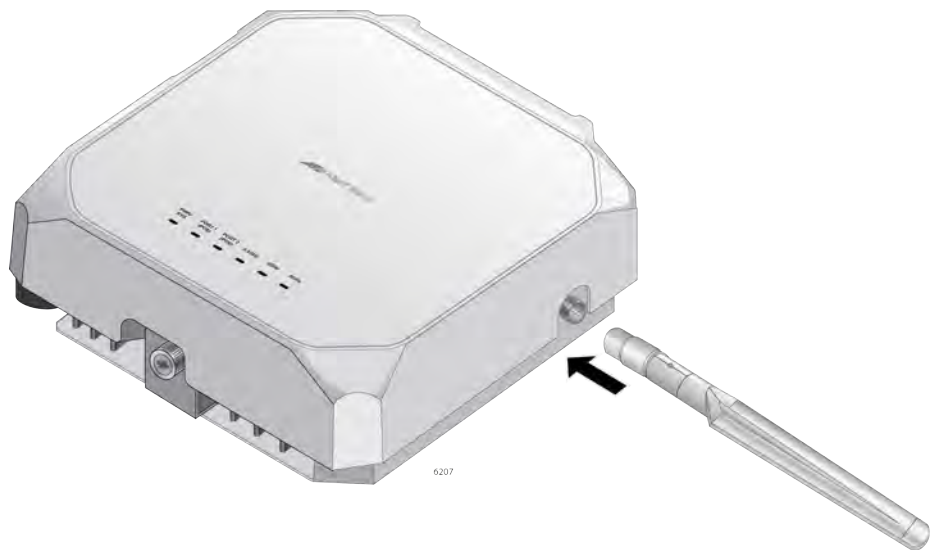
Figure 11. Aligning the Antenna to the Access Point
