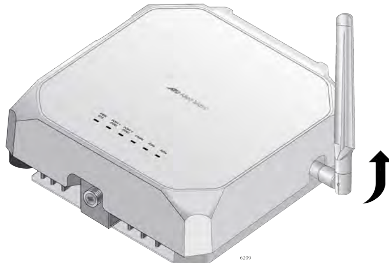
Figure 13. Adjusting the Antenna Position
