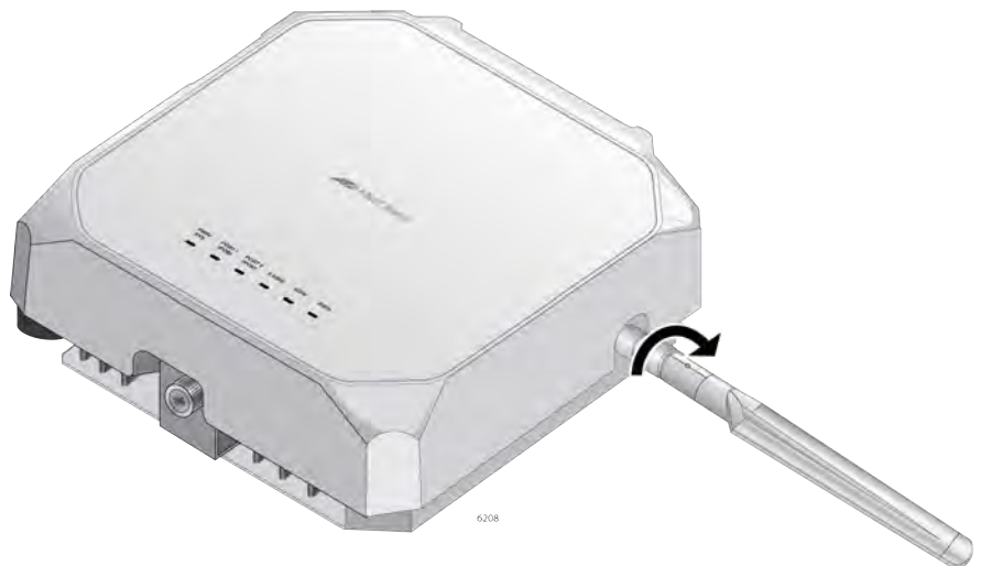
Figure 12. Attaching the Antenna to the Access Point
