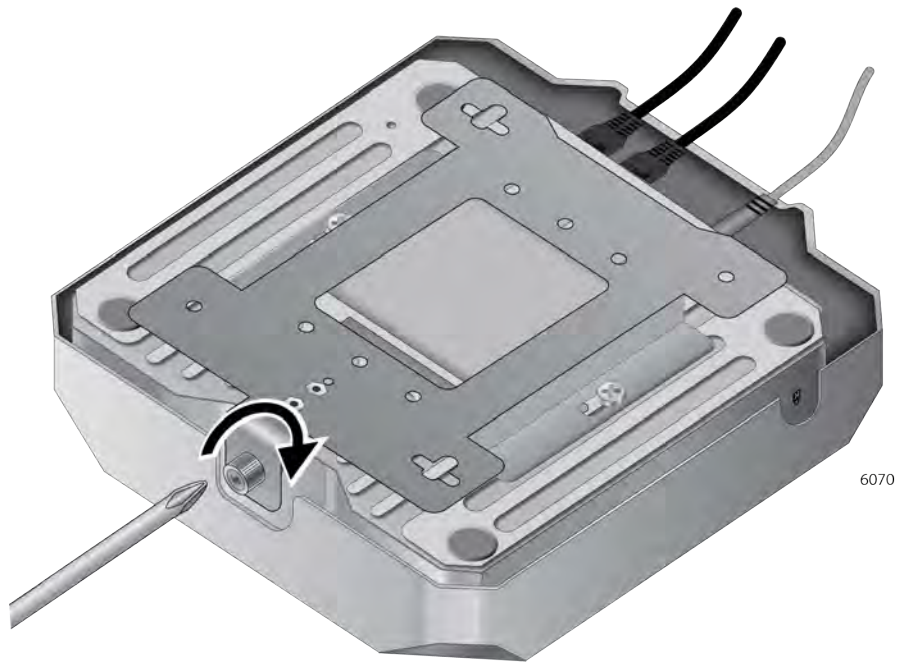
Figure 27. Tightening the Mounting Bracket Thumbscrew
