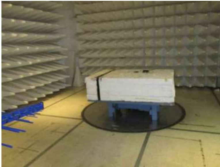
Section 7.12, Below 1GHz Test Setup
