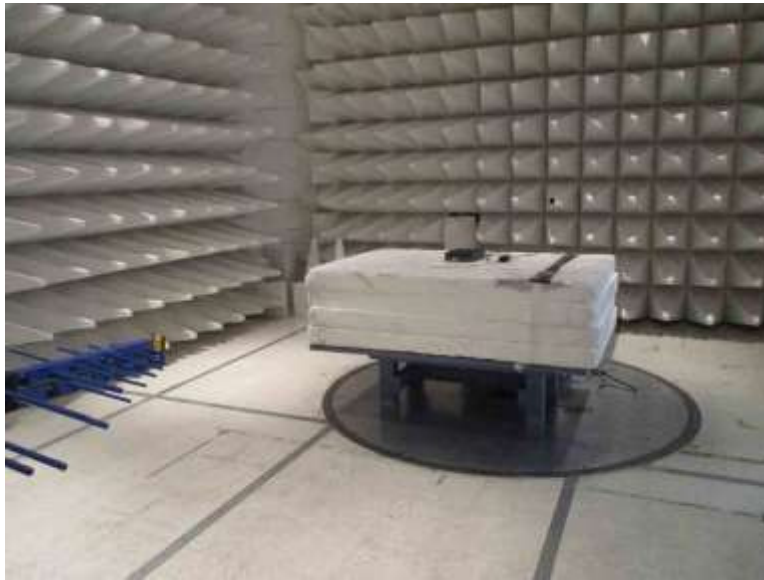
Section 7.12 Below 1GHz Test Setup
