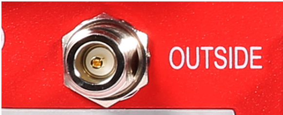
A1 — N-type Female for OUTSIDE cable and antenna
