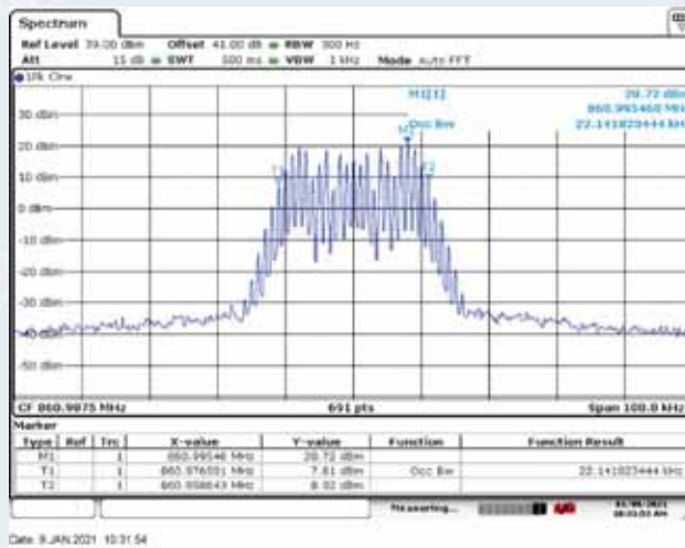
High Frequency: 860.9875MHz, Output occupied BW (with the input signal amplitude set 3 dB above the AGC threshold)
