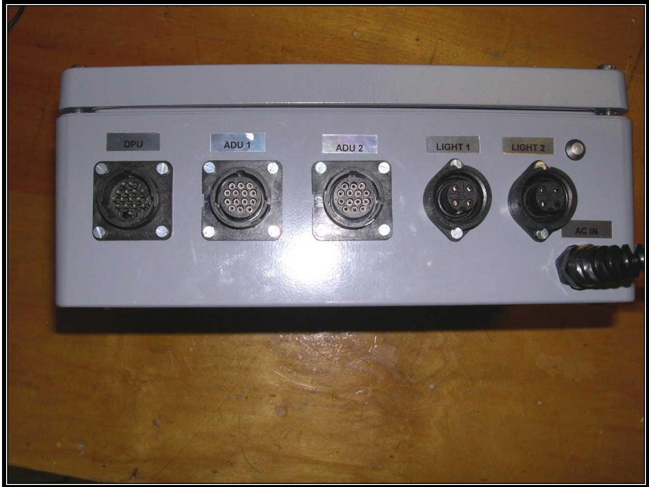
PHOTOGRAPH 19: POWER SUPPLY–FRONT VIEW
